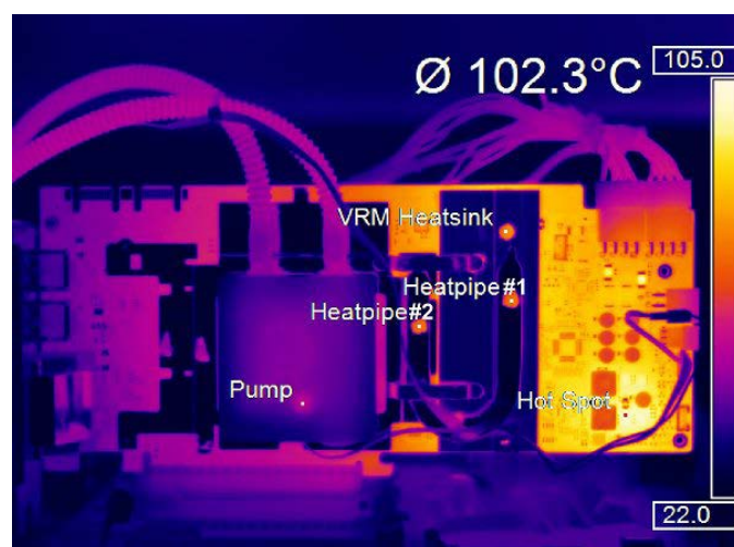
Thermal image of an operating motherboard Source: www.igorslab.de/en/ (Igor Wallossek)
